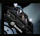
305x28 mm self-ventilated perforated brake discs Aluminum 4-pistons fixed brake calipers available colours: grey, yellow, red (standard on Competizione and Esseesse), black.
